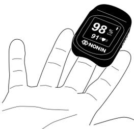
4. View about 4 seconds of readings before relying on the displayed values. Continually verify operation. It is common for the displayed values to vary slightly over a period of several seconds. If the 3230 does not turn on or if it shuts off unexpectedly:
