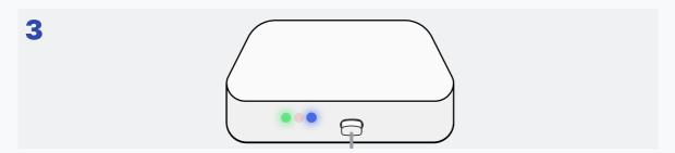
After a few minutes of blinking, the **blue** and **green** lights should become **constant**, indicating that the device is connected.
