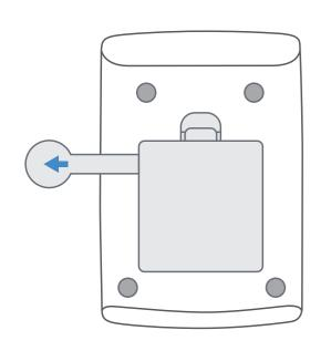
**Remove the plastic tab** from the battery compartment.
