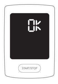
The device will display within 2 minutes if the measurement has been successfully transmitted. If not, your measurement will be stored and the device will try again following the next reading..
