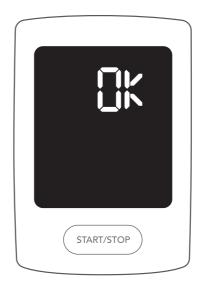
The device will display [] within 2 minutes if the measurement has been successfully transmitted. If not, your measurement will be stored and the device will try again following the next reading.
