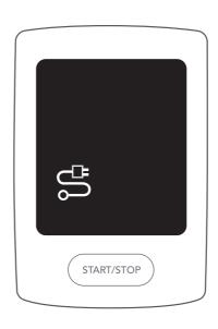
Ensure you push the cuff connector all the way in until it's fully seated in the slot. If not properly connected, the device may display an error.
